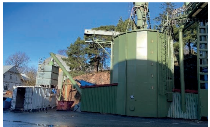
The picture shows a dust silo with a modified transport system, resulting in fewer briquettes for incineration.
